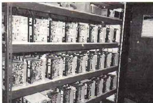
Right: HF-225 chassis, in from the subcontractors, undergo a lengthy period of soak testing before being tested, aligned and finished off.
